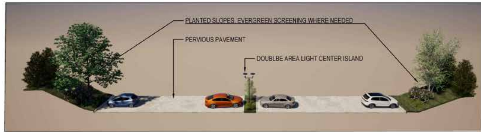
1 SCHEMATIC PARKING SECTION A-B NOT TO SCALE
