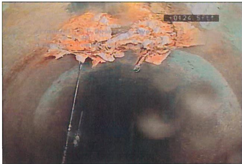
Photo: 179_180_1055_A.JPG, VCR No.: disc #18 124.5FT, Infiltration Runner, at 11 o'clock, within 8 inches of joint: YES
