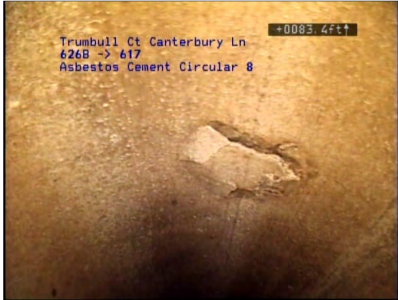
Photo: 155_155_856_A.jpg, VCR No.: Disc 12 83.4FT, Broken, from 12 to 01 o'clock, within 8 inches of joint: NO
