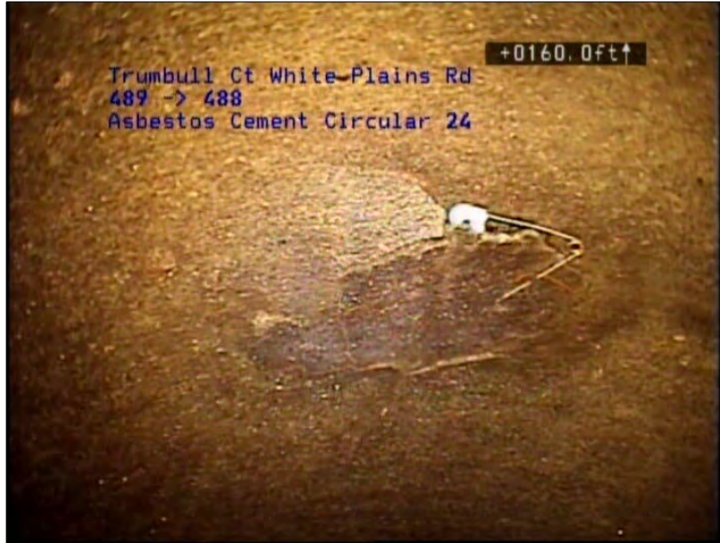
Photo: 452_452_2306_A.jpg, VCR No.: 39 160FT, Broken, from 12 to 01 o'clock, within 8 inches of joint: NO
