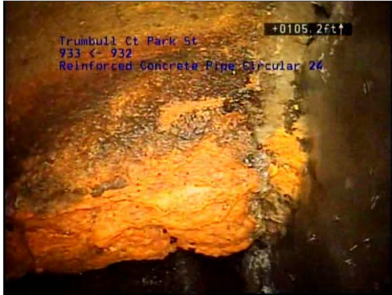
Photo: 497_497_2501_A.jpg, VCR No.: 44 106FT, Infiltration Runner, from 03 to 05 o'clock, within 8 inches of joint: NO
