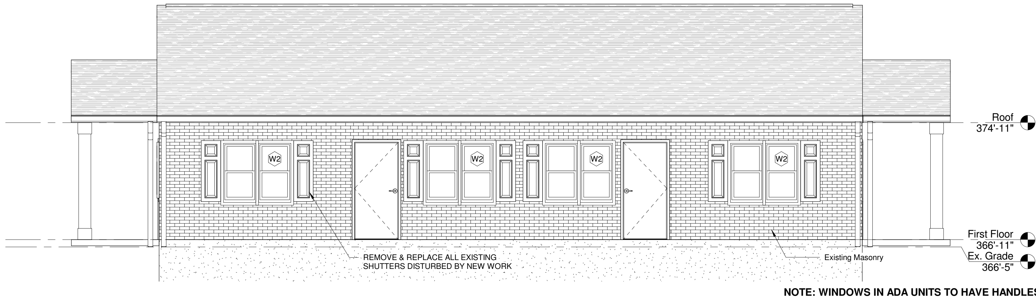
3 "Building A1" North & South Elevations Scale: 1/4" = 1'-0"
