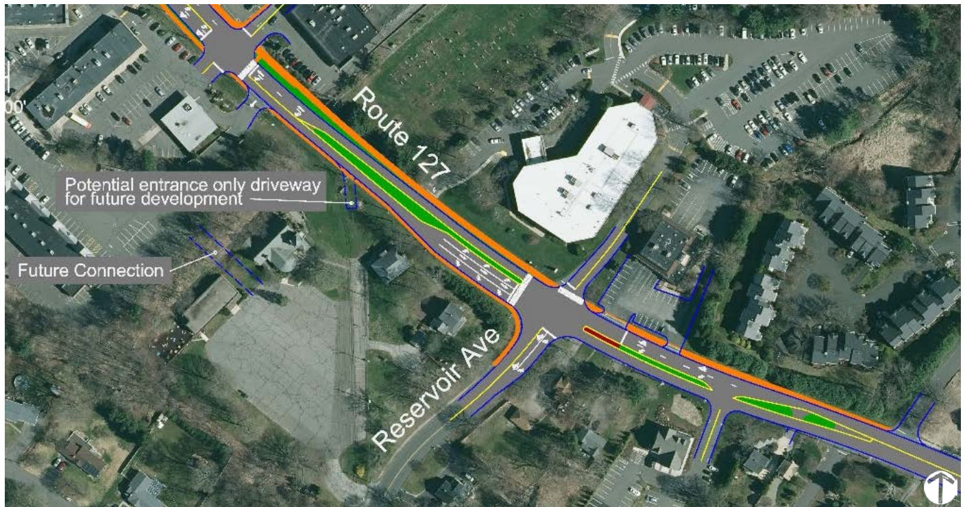
Proposed roadway and sidewalk improvements for the southern end of the Trumbull Center Corridor. Proposed sidewalks and a 10' wide multi-use trail are shown in orange. Proposed medians are depicted in bright green.
